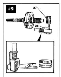
Remove the mode shift sleeve (27) and mode fork assembly (25) from the mainshaft. Note position of the mode sleeve in the fork and remove the sleeve.
